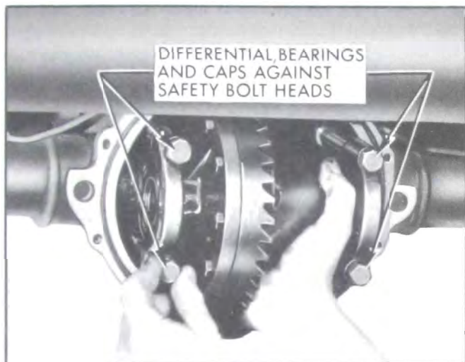
Figure 6-12—Differential Assembly Supported by Safety Bolts
