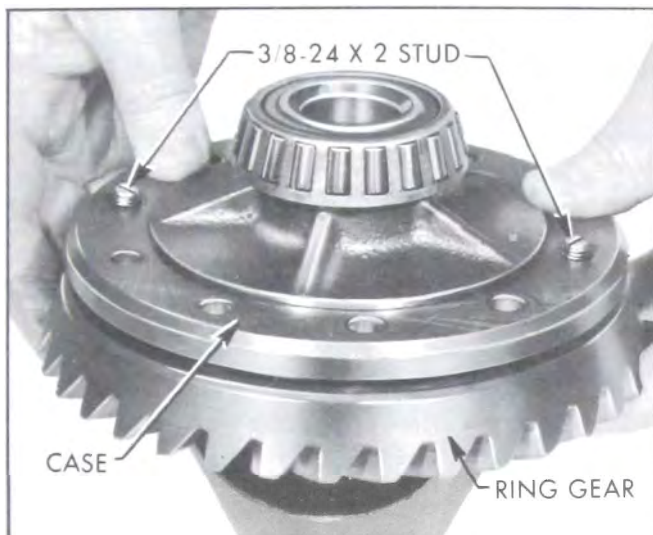
Figure 6-18—Installing Ring Gear on Differential Case
