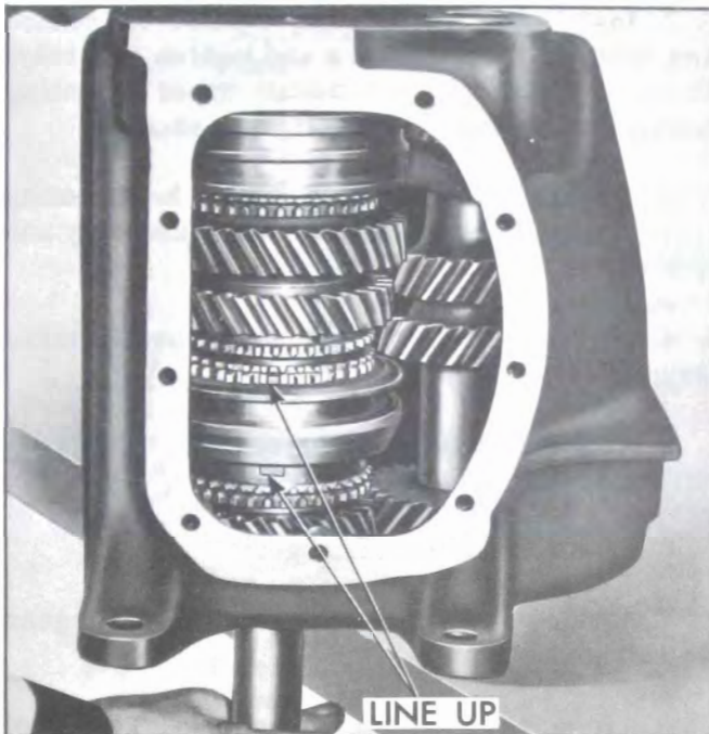
Figure 4-66—Installing Mainshaft Assembly
