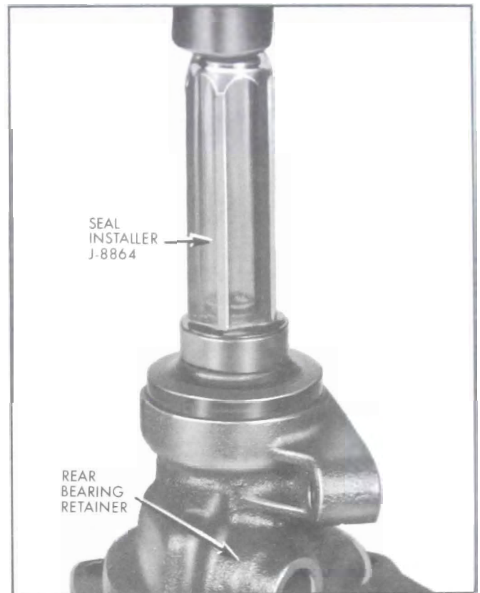
Figure 4-33A—Installing Rear Bearing Retainer Oil Seal
