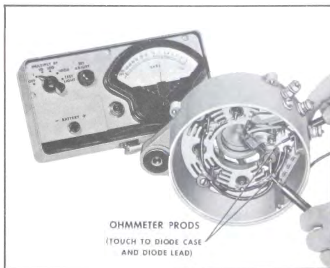
Figure 10-82—Checking Diodes
