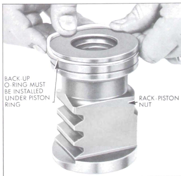
Figure 8-51—Installing Piston Ring on Rack-Piston Nut
