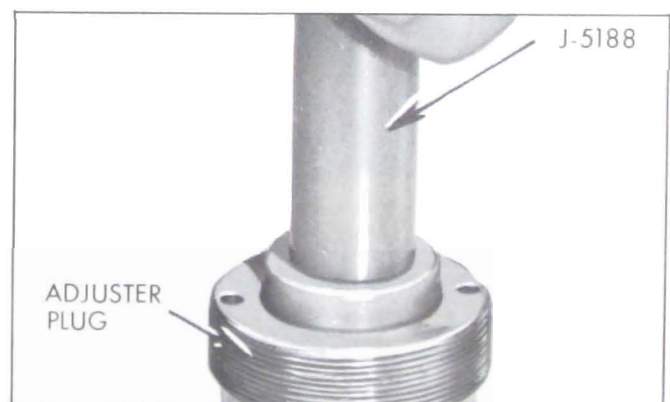
Figure 8-34—Installing Stub Shaft Seal
