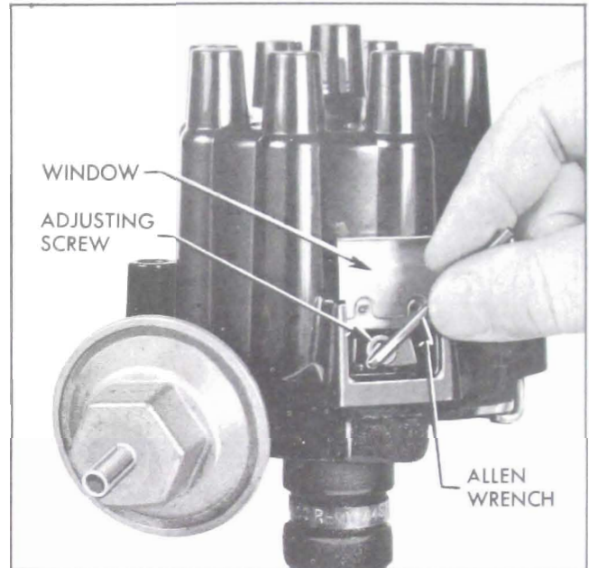
Figure 10-38—Adjusting Contact Point Dwell Angle
