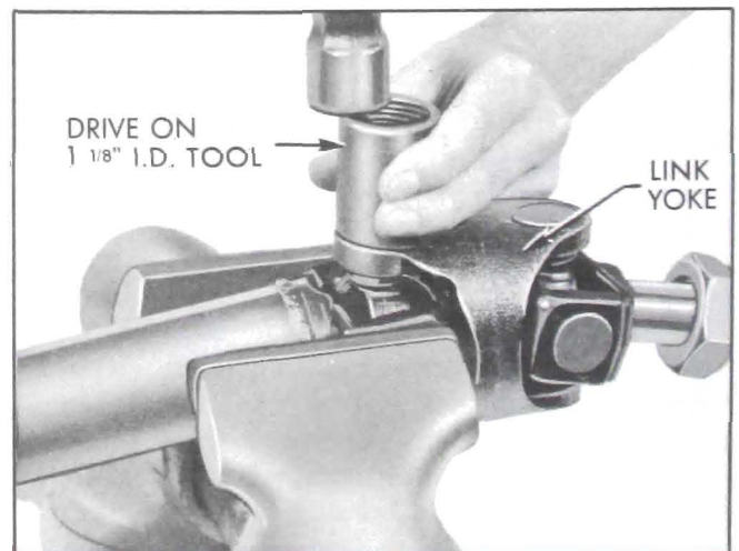
Figure 6-35—Driving Universal Joint Bearing from Link Yoke
