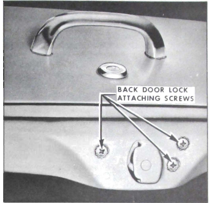
Figure 13-81 — Back Door Lock Assembly Removal
