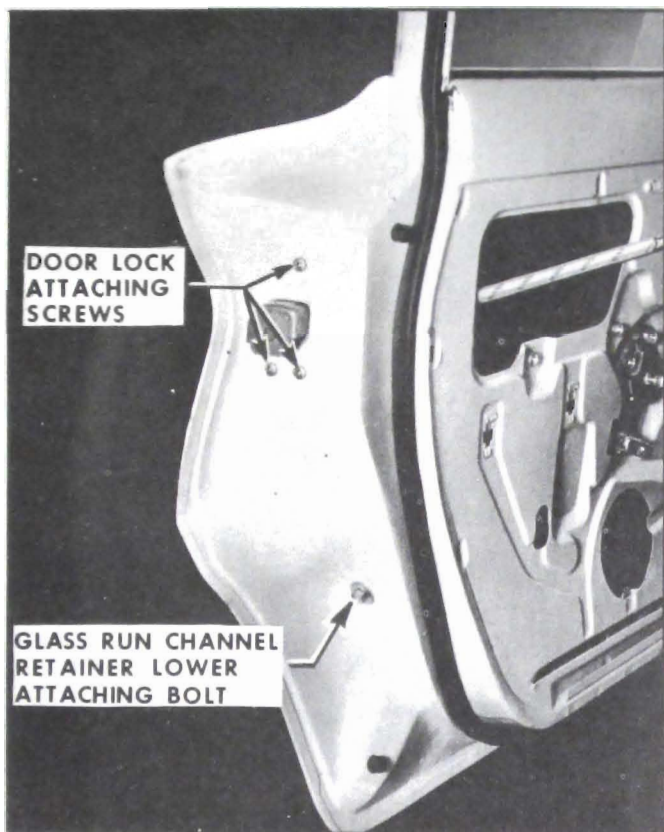
Figure 13-49—Rear Door and Glass Run Channel Retainer
