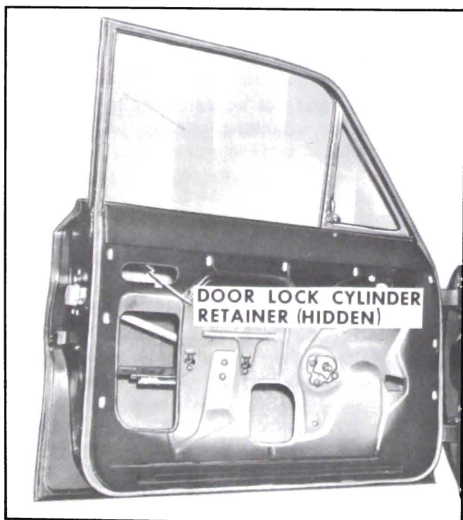
Figure 13-45—Door Lock Cylinder Attachment
