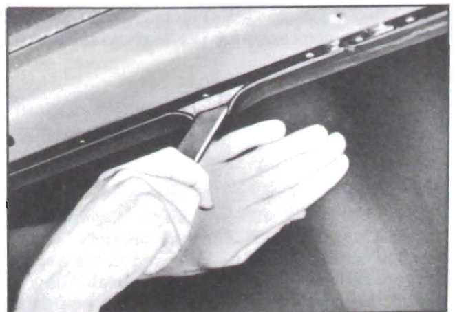
Figure 13-3—Windshield Glass Removal
