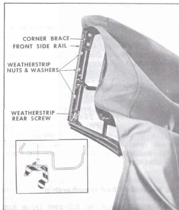
Figure 7-16—Side Roof Rail Weatherstrip
