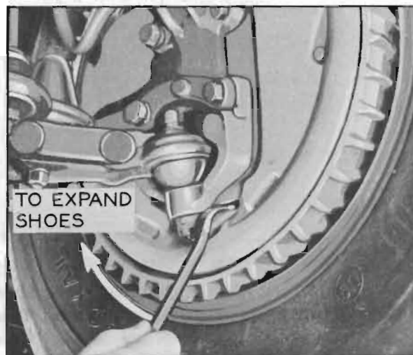
Figure 9-7—Expanding Brake Shoes
