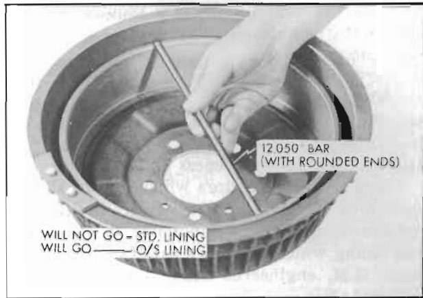
Figure 9-9—Measuring Brake Drum Size
