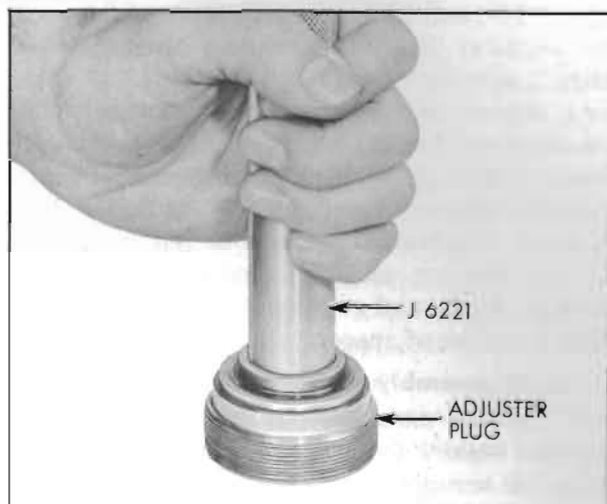
Figure 8-32—Removing Needle Bearing
