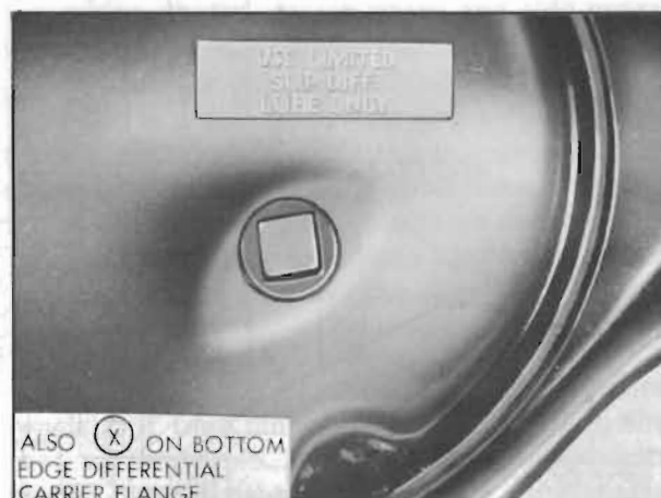
Figure 6-39—Identification of Positive Traction Differential Axle
