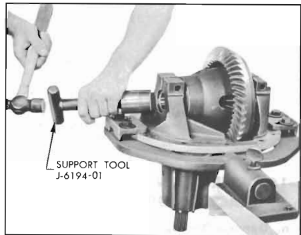
Figure 6-36—Installing Differential Bearing Supports
