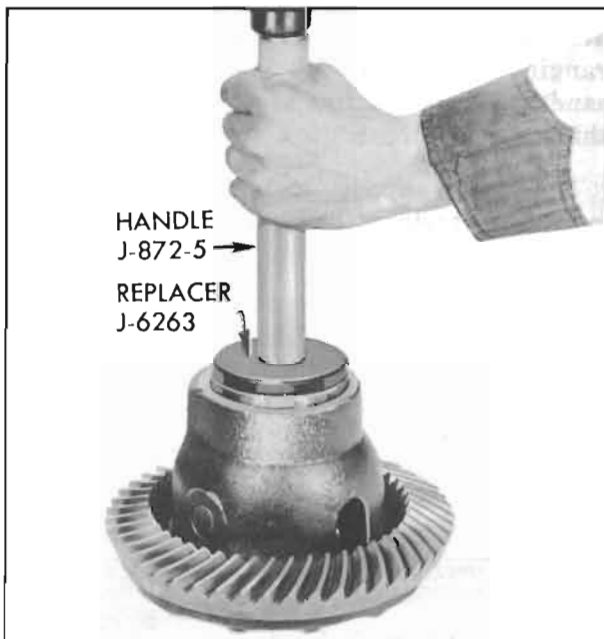
Figure 6-31—Installing Differential Bearing Outer Race
