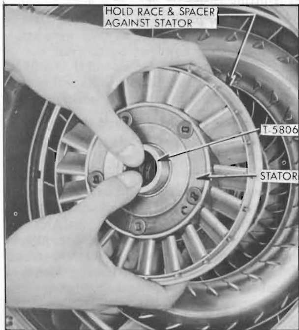
Figure 5-29—Removing Stator Assembly
