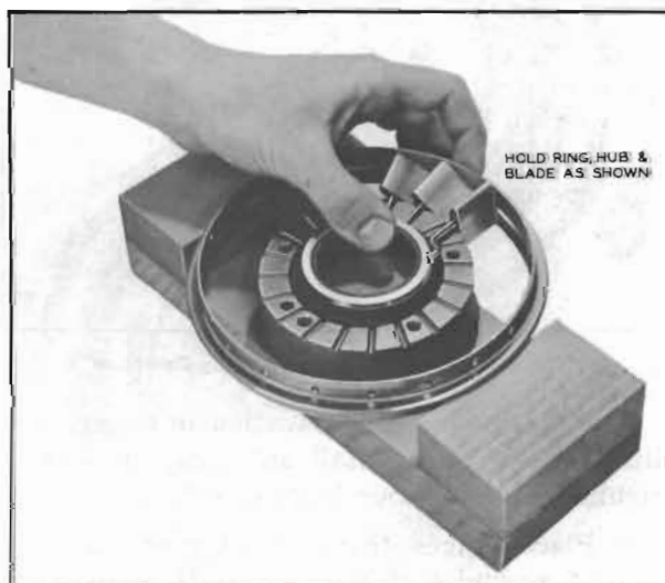
Figure 5-55—Inserting Stator Blades in Carrier
