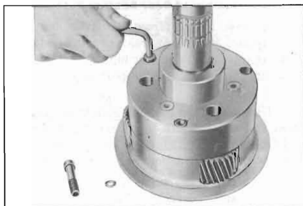
Figure 5-90—Removing Planet Carrier Screws
