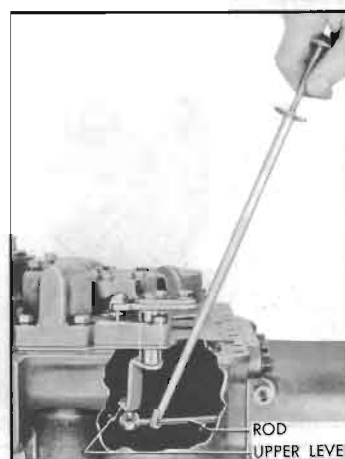
Figure 5-109—Connecting Valve Operating Rod to Upper Lever
