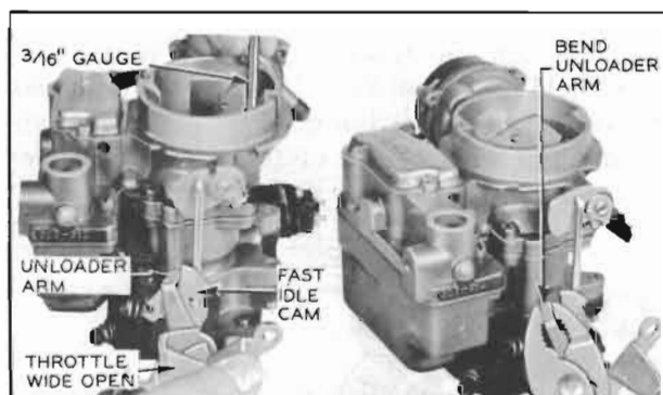
Figure 3-28—Choke Unloader Adjustment
