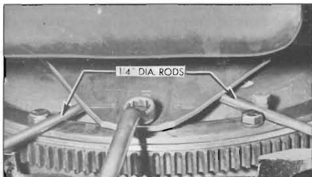
Figure 2-46—Bending Flywheel Leg Toward Pump Cover
