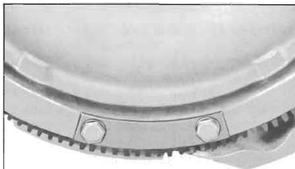
Figure 2-47—Installation of Balance Weight
