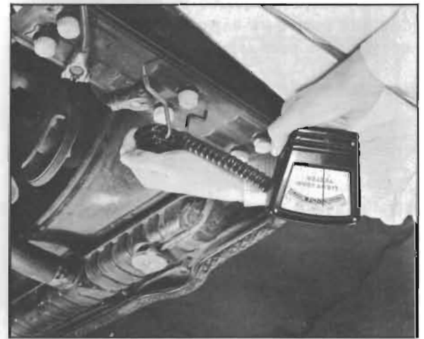
Figure 10-3—Light Load Test
