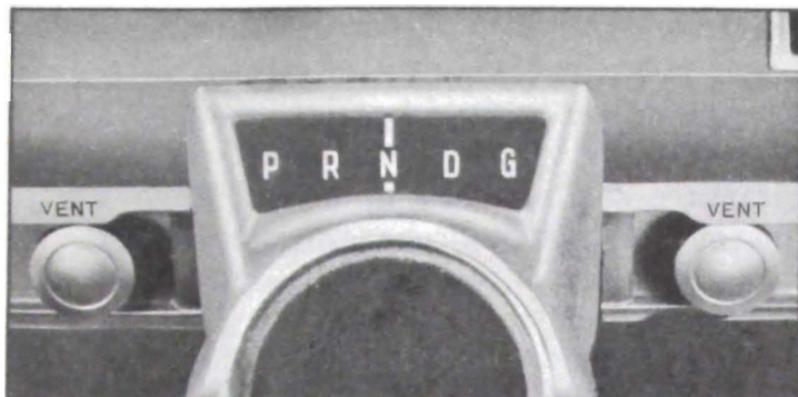
Figure 11-10—Outside Air Vent Controls
