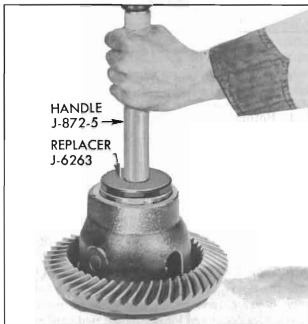
Figure 6-33—Installing Differential Bearing Outer Race
