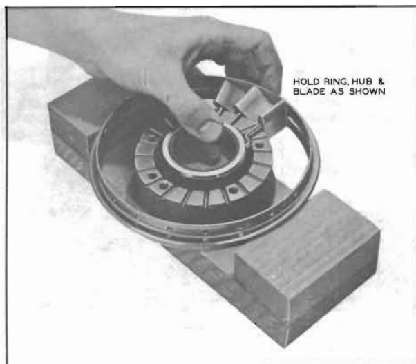
Figure 5-53—Inserting Stator Blades in Carrier
