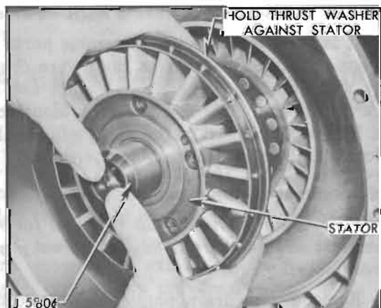
Figure 5-29—Removing Stator Assembly
