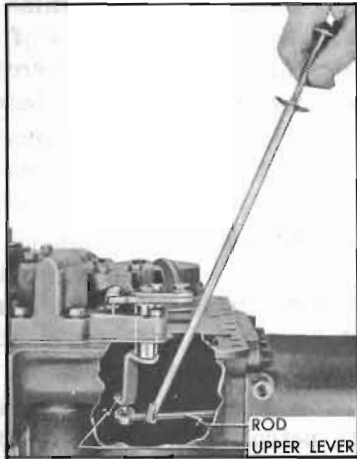
Figure 5-101—Connecting Valve Operating Rod to Upper Lever
