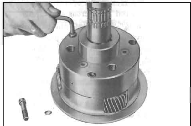
Figure 5-82—Removing Planet Carrier Screws
