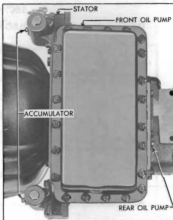
Figure 5-26—Gauge Connections for Oil Pressure Tests
