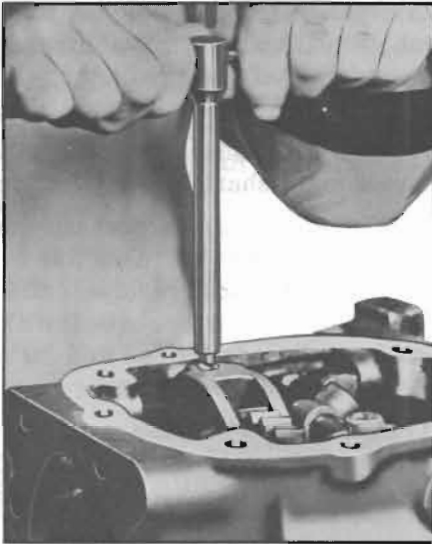
Figure 4-19—Removing Set Screw with Remover J-2895
