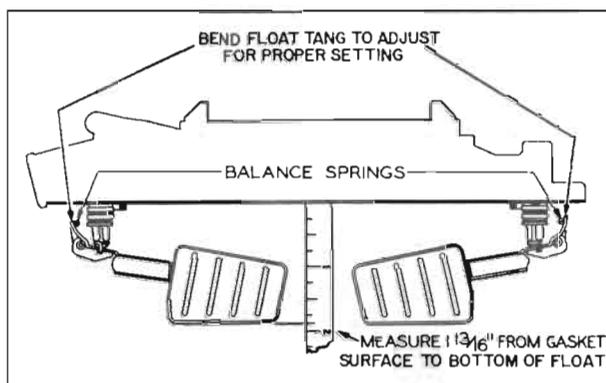
Figure 3-95--Float Drop Adjustment
