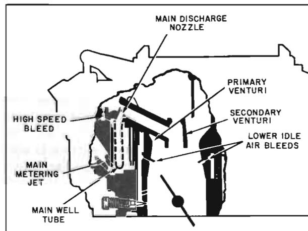
Figure 3-78—Primary Main Metering System
