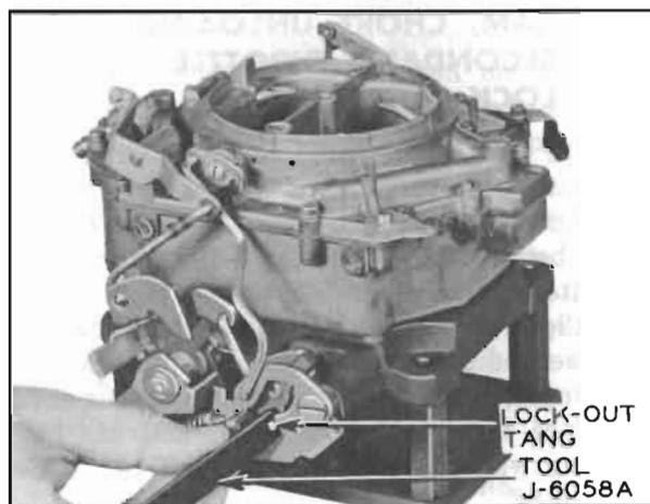
Figure 3-89—Adjusting Secondary Contour
