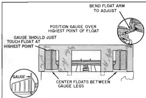
Figure 3-93--Float Level Adjustment
