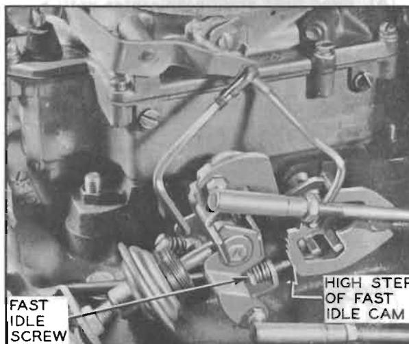
Figure 3-98—Adjusting Fast Idle
