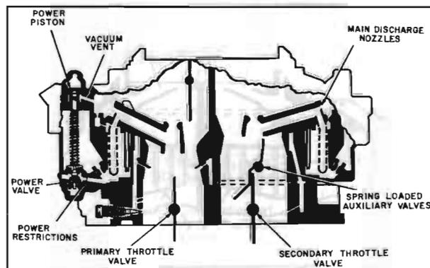
Figure 3-79—Main Metering and Power Systems
