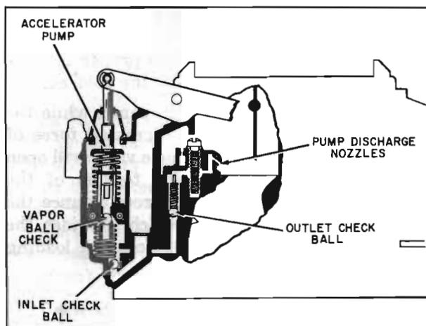
Figure 3-80—Accelerating System
