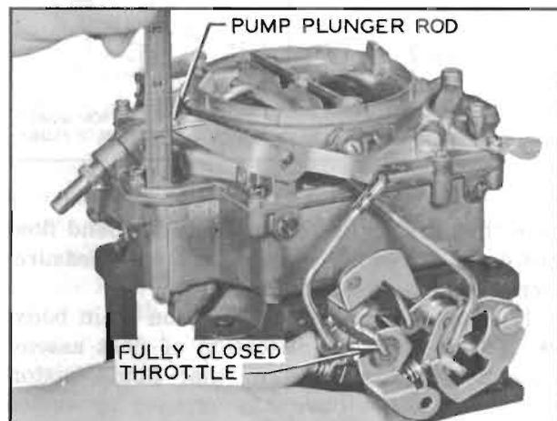
Figure 3-96—Checking Pump Plunger Adjustment
