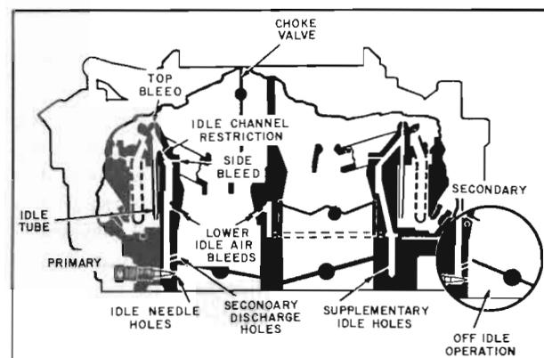
Figure 3-77—Primary and Secondary Idle Systems
