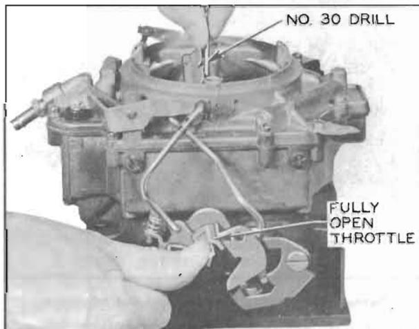
Figure 3-84—Checking Choke Unloader Adjustment
