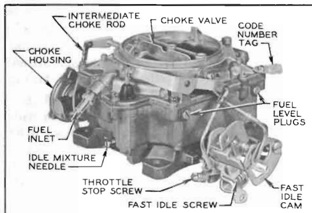
Figure 3-75—Rochester 4-Barrel Carburetor
