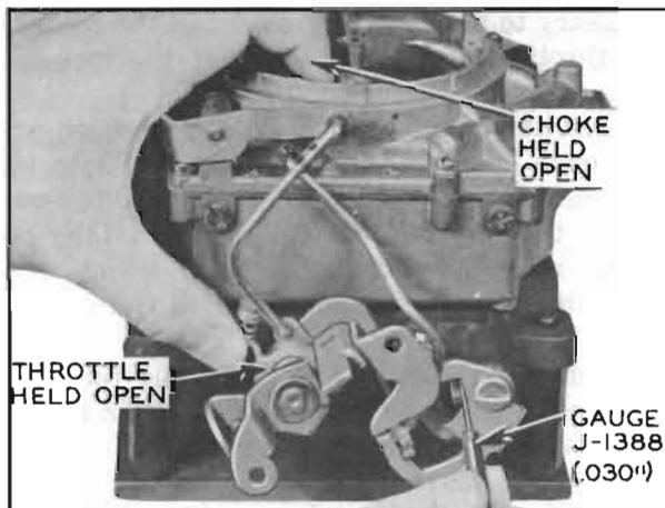
Figure 3-88—Checking Secondary Contour Adjustment
