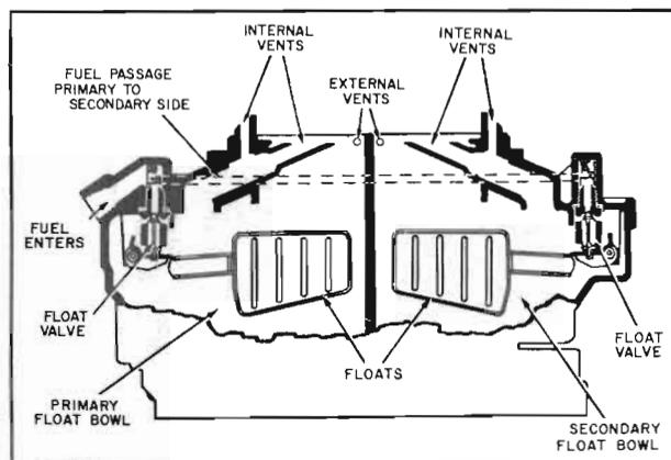
Figure 3-76—Primary and Secondary Float Systems
