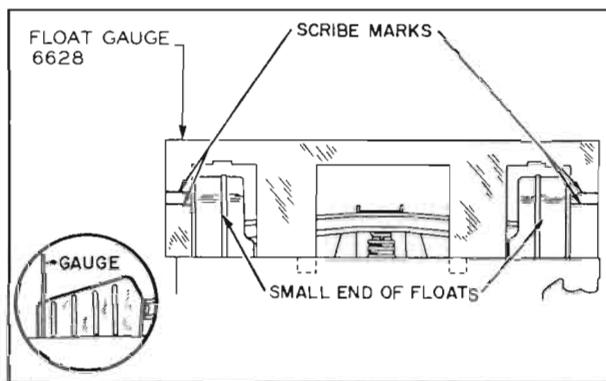
Figure 3-94--Float Tip Adjustment
