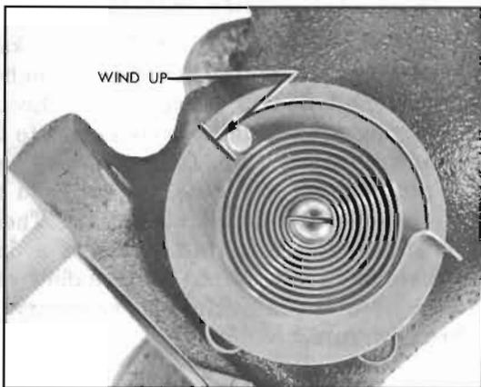
Figure 3-9—Valve Thermostat Wind-Up
