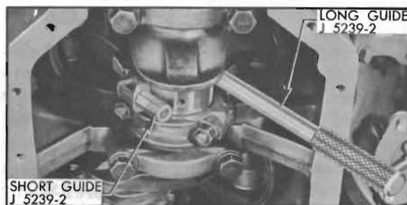
Figure 2-30—Connecting Rod Bolt Guides Installed
