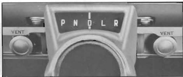
Figure 11-13—Outside Air Vent Controls
