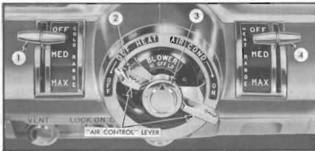
Figure 11-22—Air Conditioner Controls
