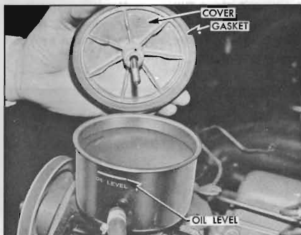
Figure 1-6—Oil Pump Reservoir
