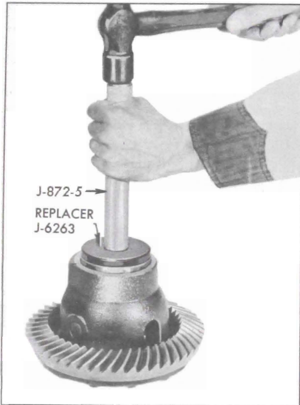
Figure 6-30—Installing Differential Bearing Outer Race
