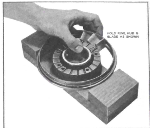
Figure 5-53—Inserting Stator Blades in Carrier
