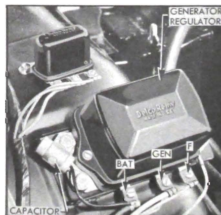
Figure 11-4—Capacitor Mounted on Generator Regulator
