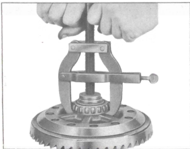
Figure 6-13—Removing Differential Bearing, Using Puller
