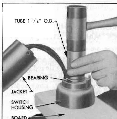
Figure 7-10—Installing Control Shaft Bearing
