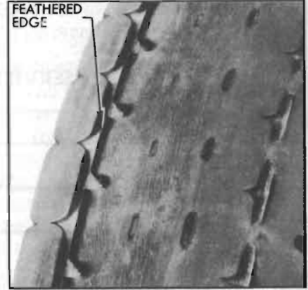
Figure 6-11—Toe-in or Toe-out Tread Wear
