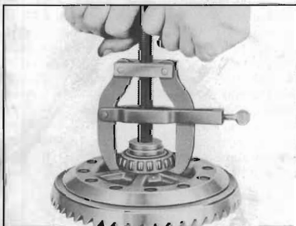
Figure 5-16—Removing Differential Bearing, Using Puller J 2241
