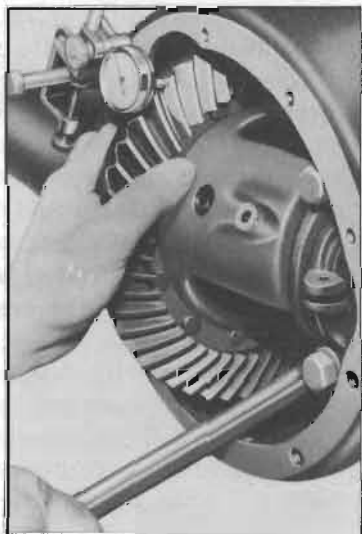
Figure 5-26—Checking Back Lash with Dial Indicator
