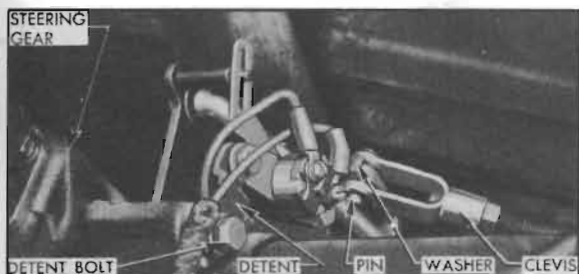
Figure 4-67—Shift Rod Adjustment
