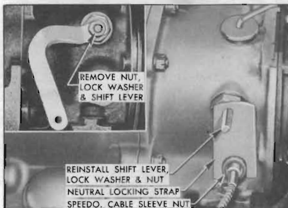
Figure 4-41—Installation of Neutral Locking Strap
