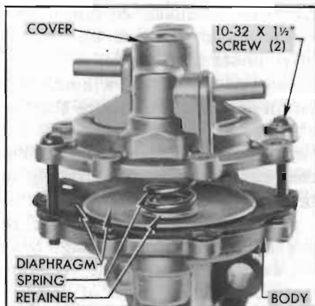
Figure 3-14—Removing Vacuum Cover
