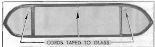
Figure 13-27—Channel and Cords Installed on Glasses
