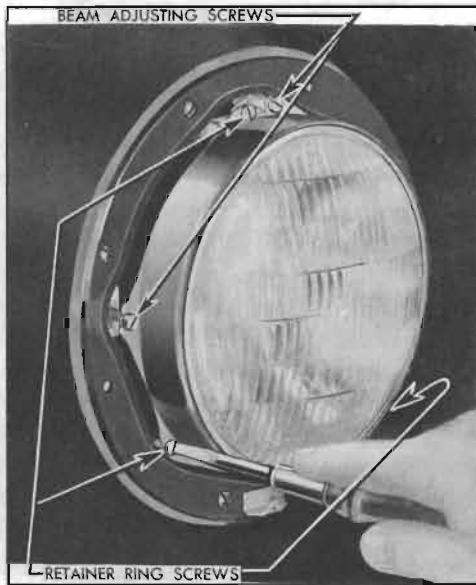
Figure 10-86—removal of Sealed Beam Unit Retainer Ring
