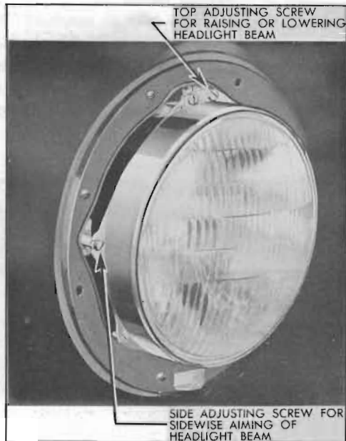
Figure 10-88—Headlamp Aiming Adjustments
