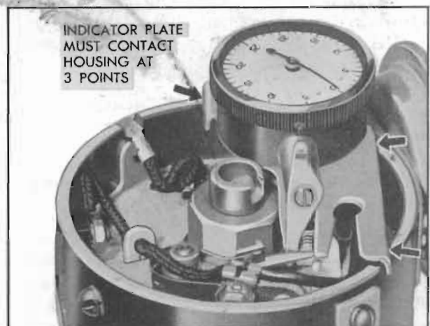
Figure 10-63—Indicator J 3955 Installed on Distributor
