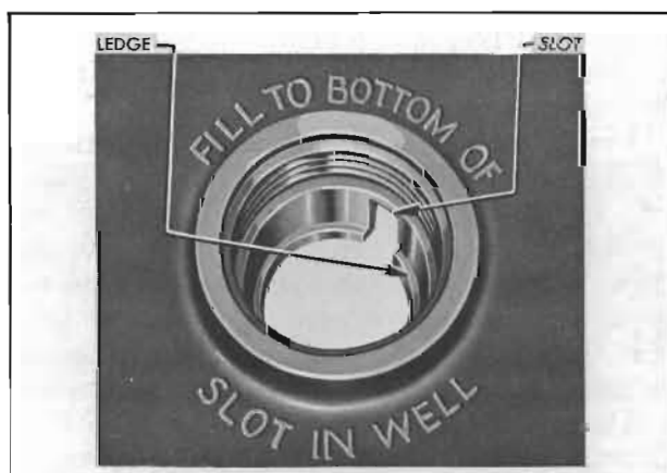
Figure 10-3—Battery Filler Well
