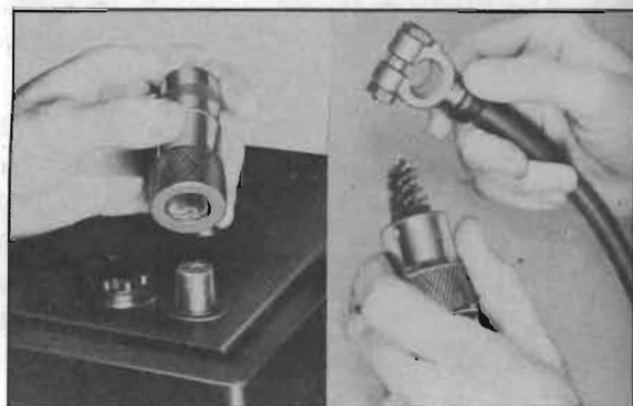
Figure 10-10—Wire Brushes for Cleaning Battery Posts and Terminals
