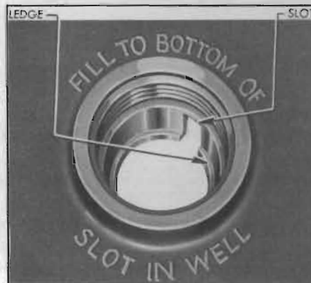
Figure 1-5—Battery Filler Well
