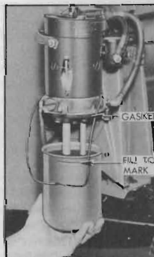
Figure 1-17—Filling H-L Power Unit Reservoir
