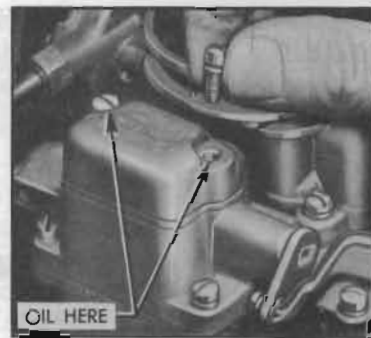
Figure 1-13—Countershaft Lubrication—2-Barrel Carter
