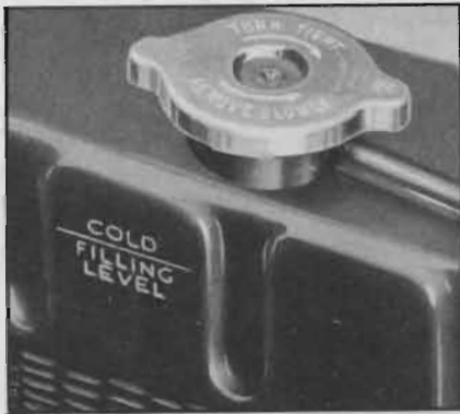
Figure 1-6—Radiator Filling Level—Cold
