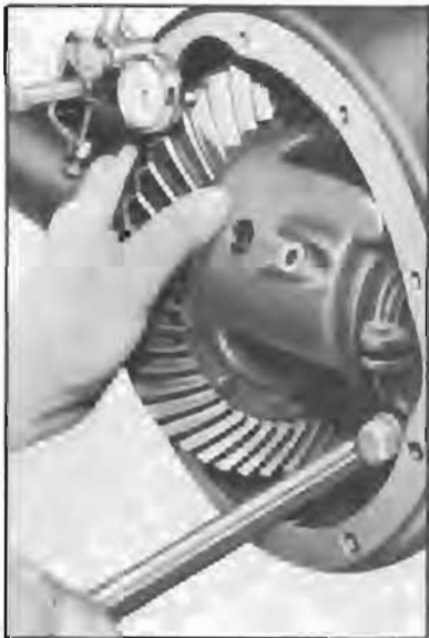
Figure 5-28—Checking Back Lash with Dial Indicator
