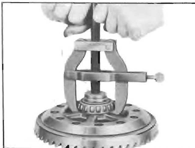
Figure 5-16—Removing Differential Bearing, Using Puller J 2241
