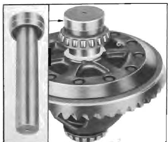
Figure 5-17—Installing Differential Bearing Using Replacer J 2242
