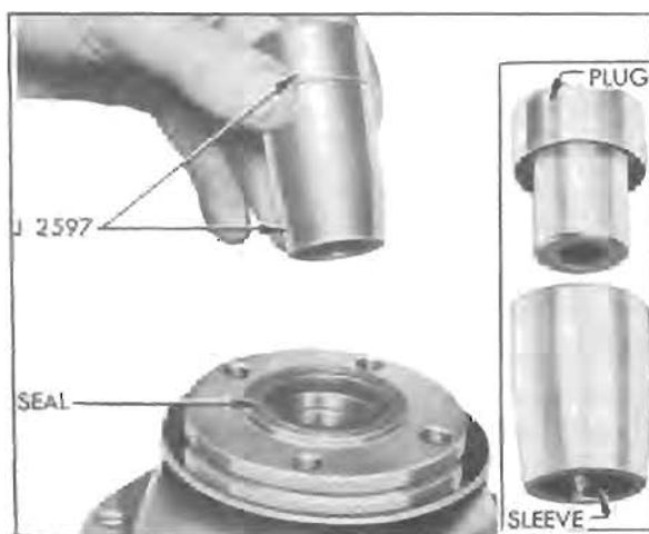
Figure 4-20—Torque Ball Installing Tool J 2597
