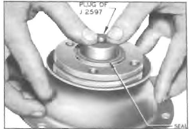
Figure 4-21—Pushing Installing Tool into Universal Joint Oil Seal
