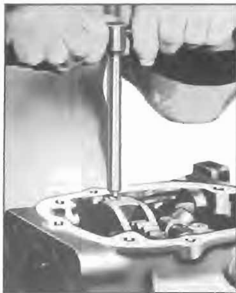
Figure 4-30—Removing Set Screw with Remover J 2895
