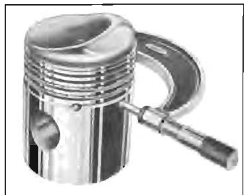
Figure 2-29—Measuring Piston with Micrometer
