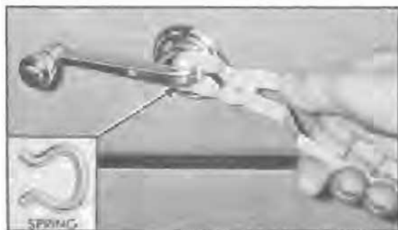
Figure 13-35—Removing Handle Retaining Spring With Pliers KMO 601
