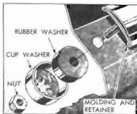
Figure 13-20—Rear Quarter Belt Molding Installation
