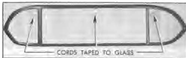
Figure 13-30—Channel and Cords Installed on Glasses
