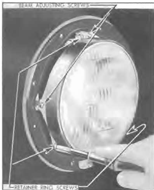
Figure 10-86—Removal of Sealed Beam Unit Retainer Ring
