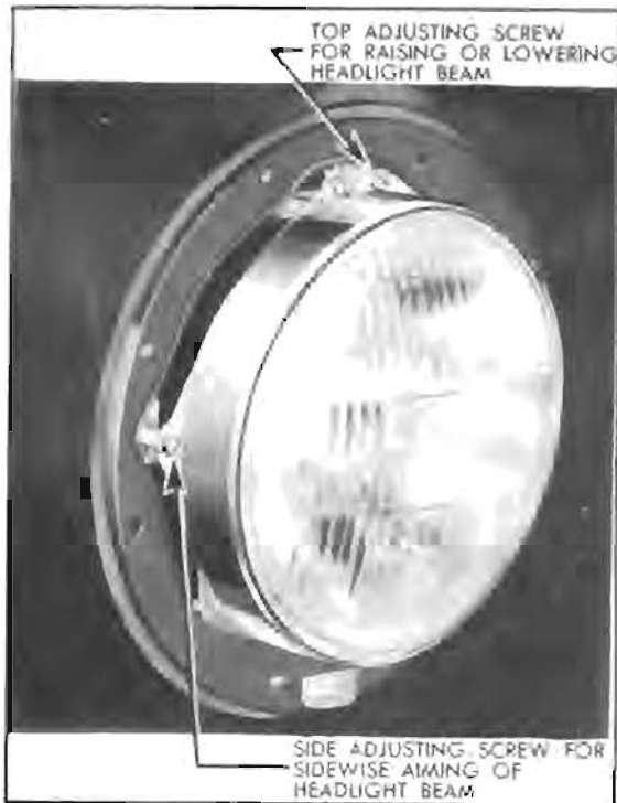
Figure 10-88—Headlamp Aiming Adjustments
