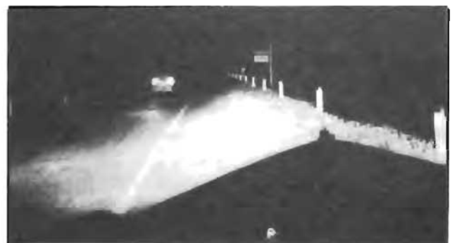
Figure 10-85—Light Distribution with Lower Headlight Beam
